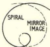
FIG. 63. THE DERIVATION OF CAM SHAPE.
